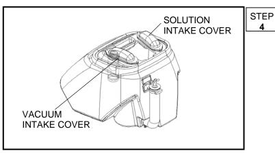
During operation, observe the following: The Cadet is equipped with clear internal covers to facilitate operator viewing of dirty solution and vacuum air flow.
